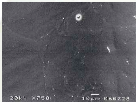
Glass-based zirconia porcelains without crystalline structures feature sensitive elasticity values and are more prone to facet-like chippings during extreme intraoral loading.
